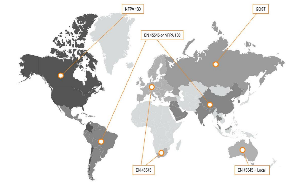
Figure 5 Schema of the international standards are of relevance in the field of materials testing
