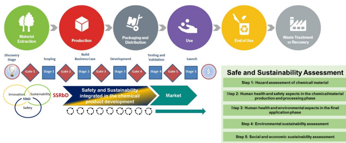
Figure 2 General life cycle thinking approach taking into account the innovation process and integrating innovation (functionality) with safety and sustainability in an iterative process.
